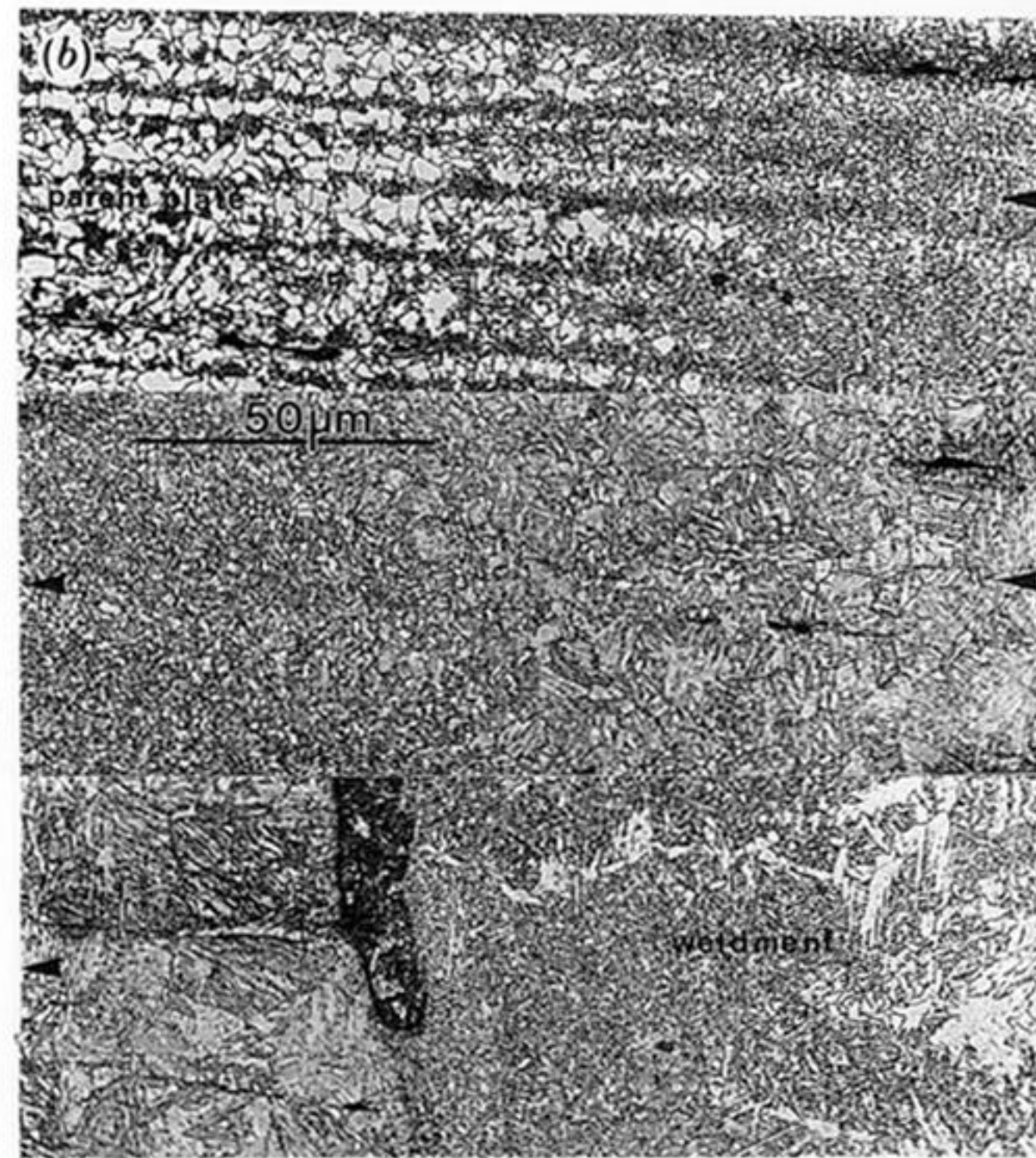
Figure 2. A light micrograph through a typical weld showing a considerable disruption in the microstructure in the heat-affected zone. This butt weld has been made by multipass manual metal arc welding in BS4360 50c plate steel. The low magnification image ( a ) reveals a number of defects in this weld arising from lack of penetration, lack of fusion, cavities and slag inclusions. The higher magnification images ( b ) reveal the disturbance to the microstructure which occurs in the heat-affected zone. The three parts of this figure ( b ) track across the heat-affected zone marked on ( a ) from the weldment to the parent plate, as shown.
