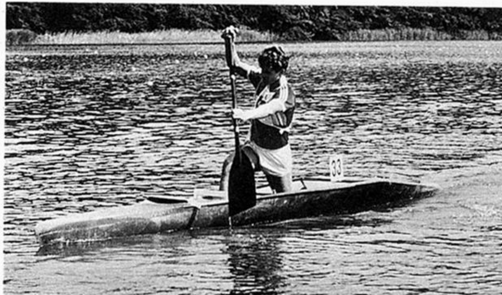
Figure 1. An example of the use of advanced materials in building small boats. In this case the total mass of the hull and paddle is under 5 kg. (Courtesy Dr Niels Hansen of the Risø National Laboratory, Denmark.)
